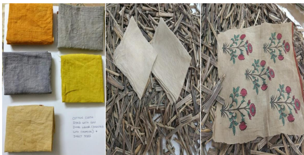
Samples of cow dung extracted liquor for making antiseptic dye for textiles
