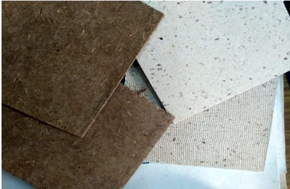
Hard board developed from cow dung and other fibers
